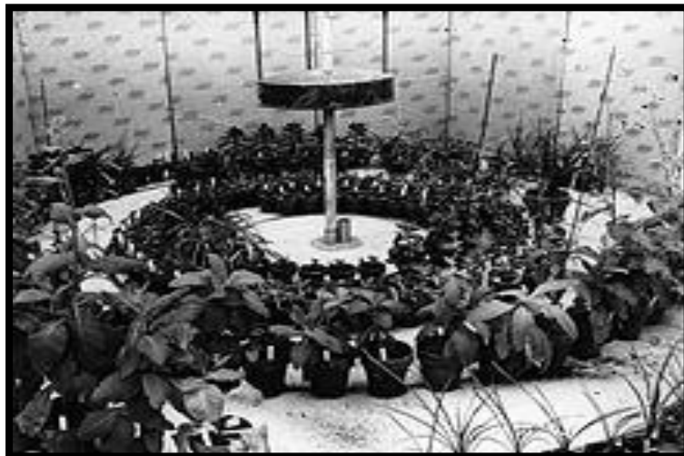
Brookhaven plant mutation experiment using ^{60}\text{Co} source in the pipe, center.
